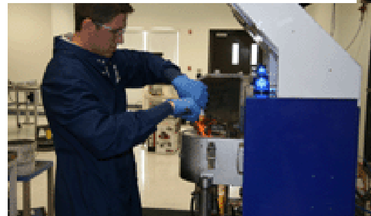
Mark Palmer, research intern, uses an induction furnace to melt samples of copper cathodes to prepare them for analysis.
